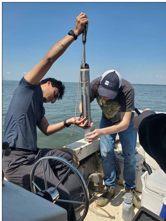
Dr. Frankel and one of his students prepare a Kemmerer water sampler, used to collect deep water samples
