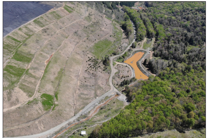
Leachate from the gob pile fouls this pond and risks groundwater contamination – Photo credit Brent Walls
